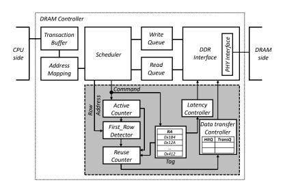
Figure 8. Implementations of in-DRAM cache manager on the DRAM controller.
