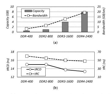
**Figure 1.** Comparison of dynamic random access memory (DRAM) capacity, bandwidth, and latency improvement by DRAM generation [4–7]. (a) Capacity and bandwidth of DRAM. (b) DRAM access latency: row address to column address delay (*tRCD*) and row cycle time (*tRC*).
